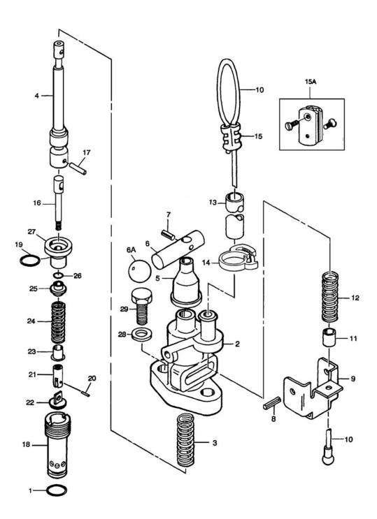
FIGURE 5 - LANYARD OPERATED PILOT VALVE
