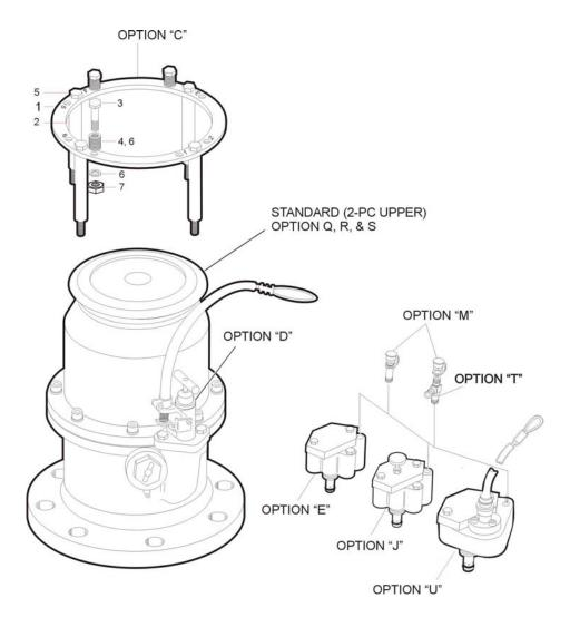
FIGURE 1 - 61654 SERIES HYDRANT VALVE OPTIONS
